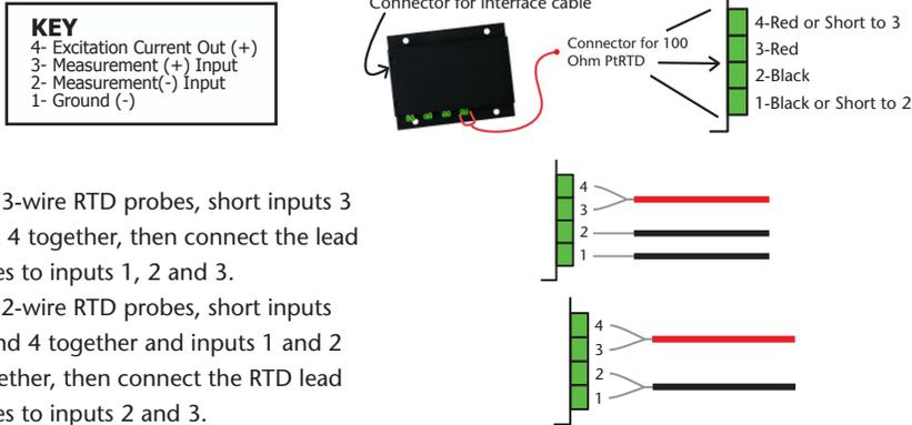
*Warning: Note the polarity instructions. Do not attach wires to the wrong terminals. 100 Ω, 2 or 4 wire RTD probes are recommended for the most accurate performance. Most 100 Ω, 3 wire RTD probes will work, but MadgeTech cannot guarantee the accuracy. To determine whether or not the 3-wire RTD probe will work, the resistance between the two same colored wires should be less than 1 Ω. (Note: Please contact the manufacturer of the RTD probe for questions on the resistance)*
